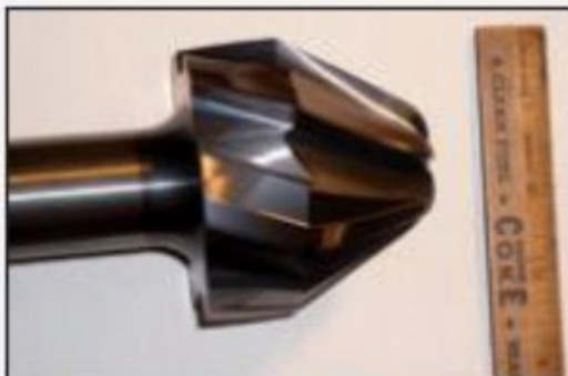
4-1/2" Dia 1-1/4" shank multi radius Carbide round tool
